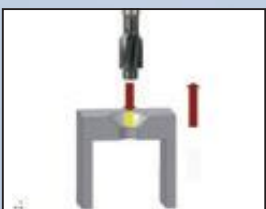
Avellanar, chaflanar Counter sinking, Facing
