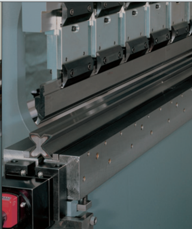
Anti deflection table for system-dies.
